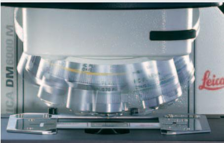
Each time an objective is changed, the illumination manager correctly determines the best parameters for the aperture and field diaphragm.
