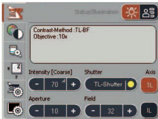
The new, external Leica STP6000 SmartTouch Panel provides convenient, remote control of all of the microscope's automated functions. It provides the same graphical user interface as LAS software.
